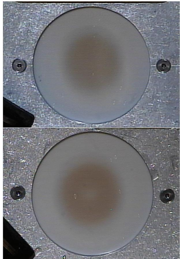
Figure 3: Beam spots at the IPF target produced using the concentric circle (top) and spiral (bottom) raster patterns measured by film irradiation.
