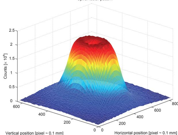
Figure 5: The beam spot at the IPF target measured by foil irradiation for the concentric circle (top) and spiral (bottom) raster patterns.
