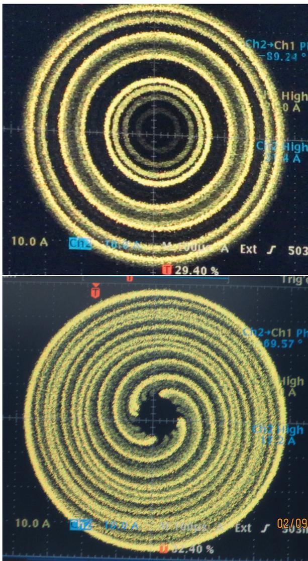
Figure 2: The raster amplitude waveforms observed by current viewing coils at the raster steering magnets for the concentric circle (top) and spiral (bottom) patterns with oscilloscope persistence for several macropulses.
