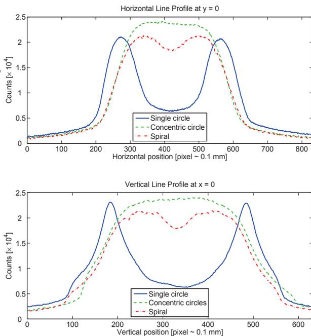
Figure 4: The horizontal (top) and vertical (bottom) beam spot line profiles at the IPF target measured by foil irradiation for single circle production (blue), concentric circle (green), and spiral (red) raster patterns.
