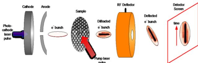
Figure 1: Overview of UED system, from photo-cathode emission on (left), through the sample, then deflector, and finally the streaked image (right).
