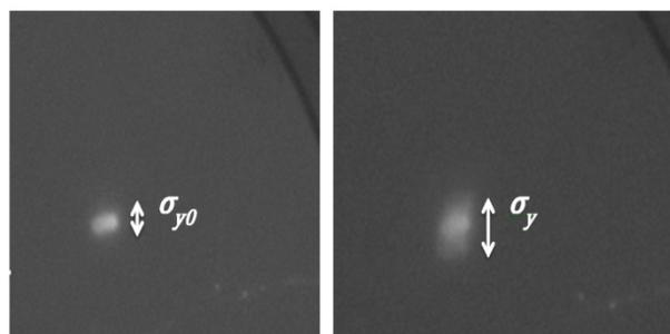
Figure 6: Beam spot as imaged with the MCP having the deflector turned off,  $\sigma_{y0} \approx 300 \mu\text{m}$  (left) and turned on,  $\sigma_y \approx 1000 \mu\text{m}$  (right).
