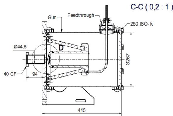
Figure 2: 100 kV electron gun employing a copper photo-cathode purchased from AccTech.
