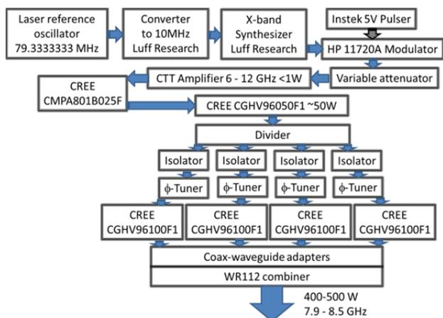
Figure 5: Simplified RF schematic for the solid-state X-band amplifier system developed for this project. DC supplies, computer control, diagnostics, and cooling systems are not shown.
