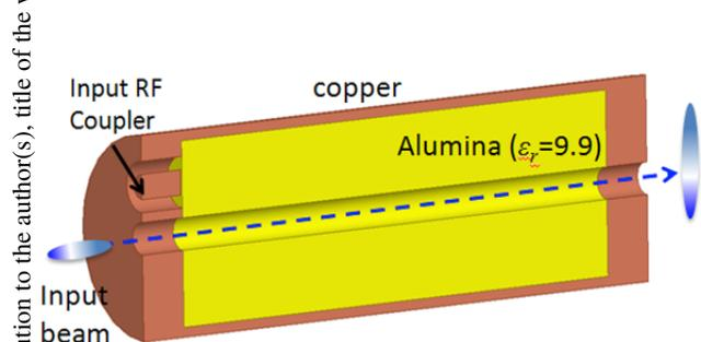
Figure 3: Model of a 6 cm long, 2 cm diameter dielectric-loaded deflector designed and fabricated for this project.
