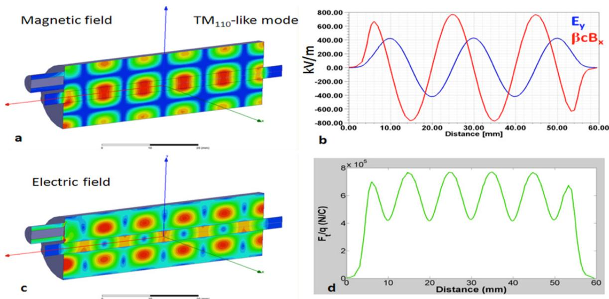
Figure 4: Simulation results from dielectric deflector showing (a) magnetic field distribution, (b) on-axis electric and magnetic components contributing to the Lorentz force, (c) electric field distribution, and (d) total Lorentz force seen by a 100 keV electron beam.
