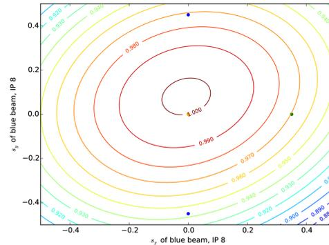
Figure 4: The luminosity reduction as a function of the  $s_H^*$  and  $s_V^*$  of the blue beam. The requested  $s_V^*$  change is marked with blue dots; the requested  $s_H^*$  is marked with green dot and the origin  $s^*$  is marked yellow dot.
