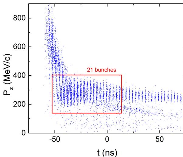
Figure 1: Longitudinal phase-space at the cooler entrance.
