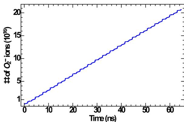
Figure 4: Number of oxygen ions as a function of time for the entire beam pulse.
