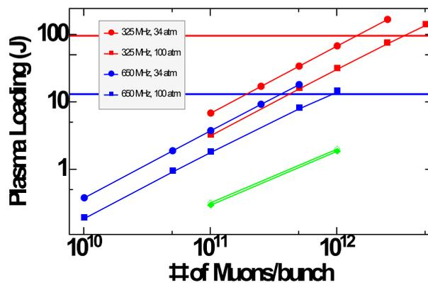
Figure 5: Total energy dissipated after the 20<sup>th</sup> bunch has passed through the cavity as a function of number of muons per bunch. The horizontal lines are the stored energy of the 325 MHz cavity (red) and 650 MHz cavity (blue). The green diamonds are the results for the Helical Cooling Channel at 180 atm, described in Ref. [7].
