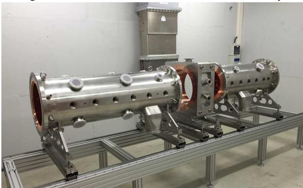
Figure 11: Prototype of coupled crossed-bar H-cavity.
