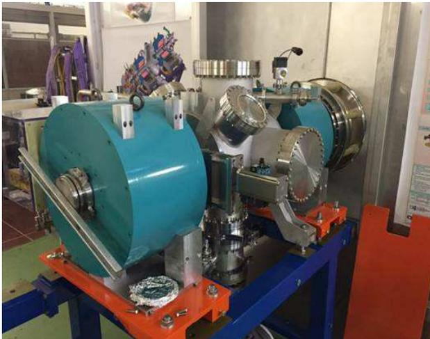
Figure 10: Proton source assembled at CEA/Saclay.
