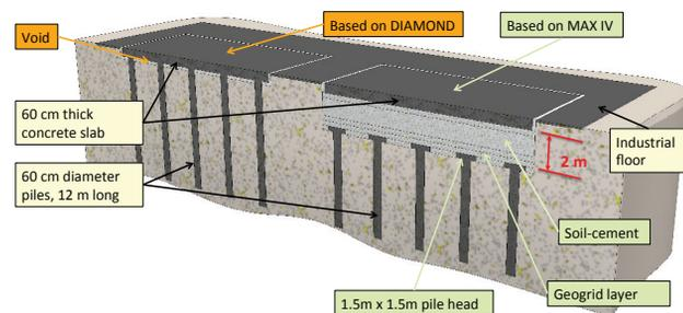
Figure 2: Two types of floor prototypes constructed at LNLs site to study and compare their performance. The concrete slab is supported exclusively on piles for the Diamond-type solution. In the MAX IV-type solution, a thick layer of soil-cement is interleaved between piles and concrete slab.
