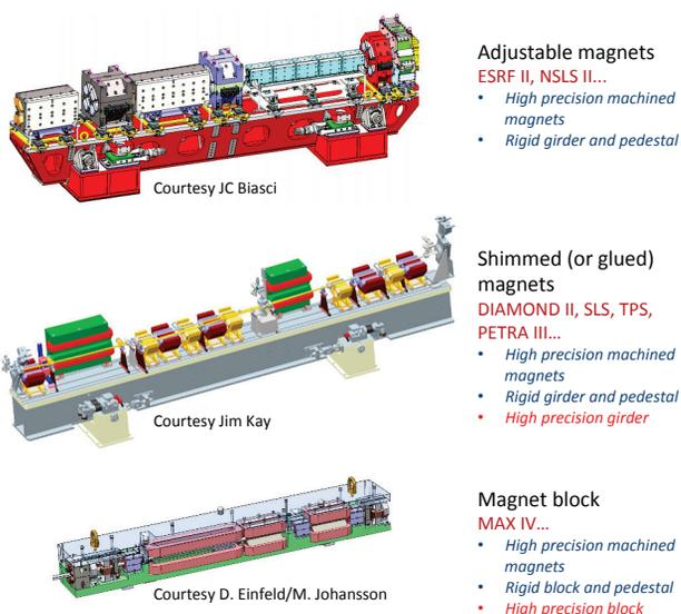
Figure 3: Different solutions adopted for magnet girders and magnet positioning systems.
