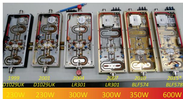
Figure 8: Evolution of the LNSL 476 MHz SSA modules showing the continuous increase of the output power over the last 15 years. The 600W module operates at 500 MHz.
