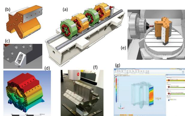
Figure 4: Proposed girder-magnet assembly for Sirius showing: (a) the girder with multipole magnets; (b) one pole of the quadrupole magnet with machine reference surfaces; (c) the designed clamping fixture; (d) structural analysis of the clamping fixture (>400 Hz vibration mode); (e) machining process developed for the quadrupole; (f) machined pole on CMM machine; and (g) results for the surface flatness measurements (< 8  $\mu\text{m}$ ).
