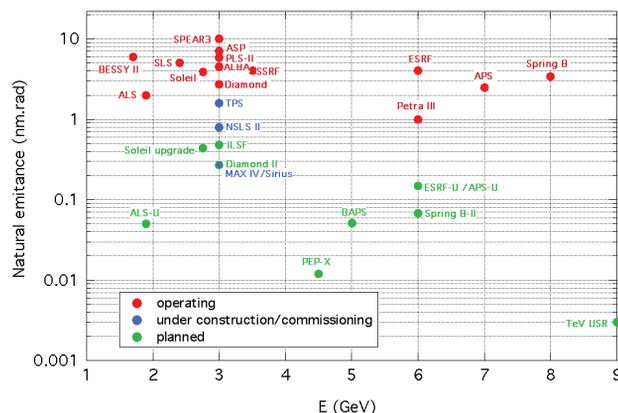
Figure 1: Survey of emittances versus energy for some existing machines that are in operation for users, for machines under construction or in commissioning phase and for some planned green-field or upgrade to existing machines.
