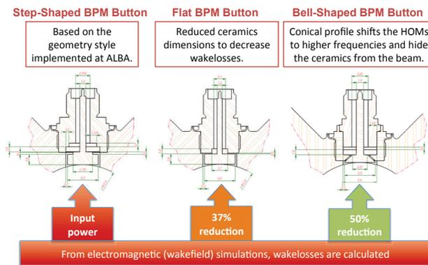
Figure 5: Effect of different button shapes and ceramic sizes on the beam power loss for the Sirius beam parameters. The buttons sensitivity is preserved in all cases.
