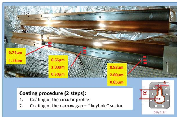
Figure 7: Development of NEG coating in a dipole chamber with a narrow (6 mm height) antechamber for radiation extraction. The picture shows the coating thickness variations for different positions inside the antechamber.
