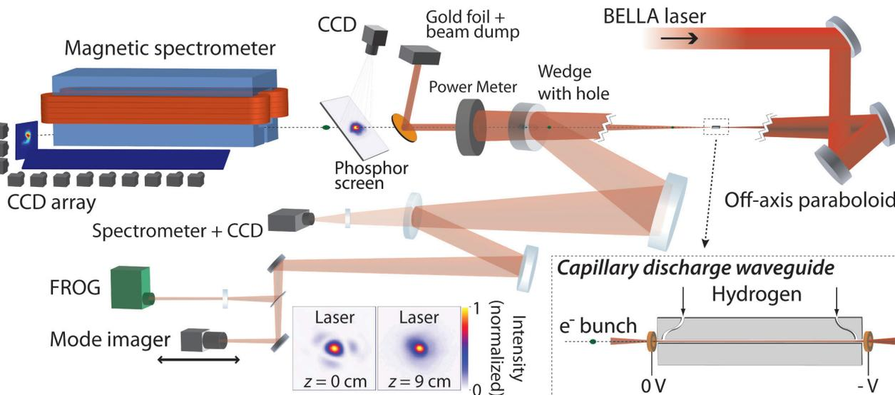
Figure 1: Schematic of the experimental setup showing the target (inset) and diagnostics of the laser and electron beam. Typical laser spatial profiles with input laser pulse energy 16.6 J are shown at focus ( $z = 0$ ) and at the exit of the capillary ( $z = 9$  cm) for density  $8 \times 10^{17} \text{ cm}^{-3}$ . The width of each image is  $500 \mu\text{m}$ .
