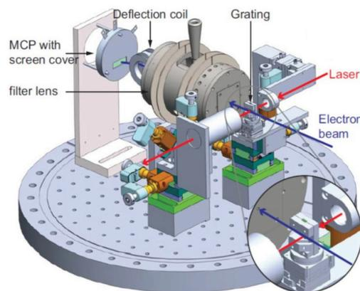
Figure 2: A schematic of the vacuum chamber used in the Erlangen DLA project. This includes the thermal emission SEM column electron source, the single grating DLA on an actuator stage, a final focusing lens for the incident laser, a microscope objective for viewing the sample from outside of the chamber, a retarding field spectrometer and a micro-channel plate detector.
