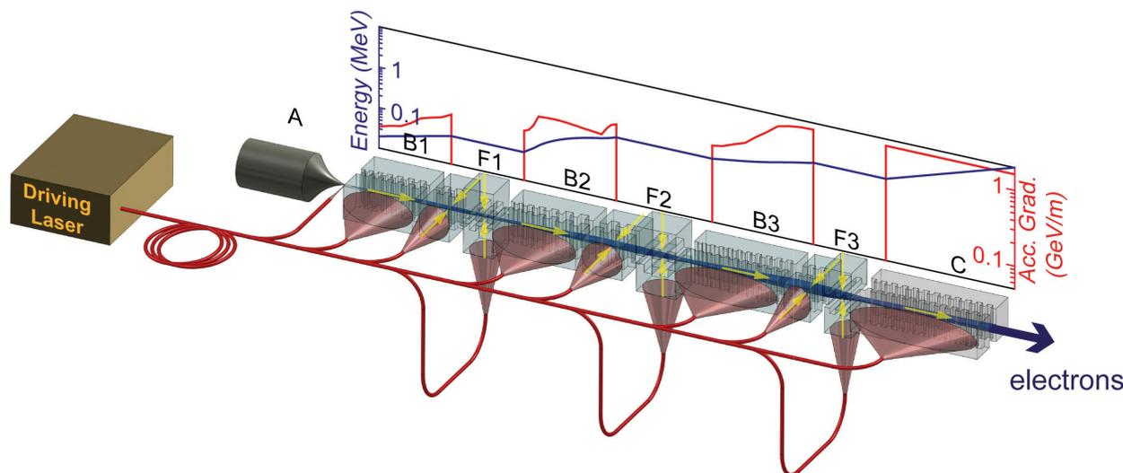
Figure 4: A schematic of an envisioned multi-stage DLA based accelerator. This includes a laser-triggered electron source, subrelativistic accelerating and focusing elements, a fiber-based laser power distribution network, and relativistic focusing and accelerating elements.
