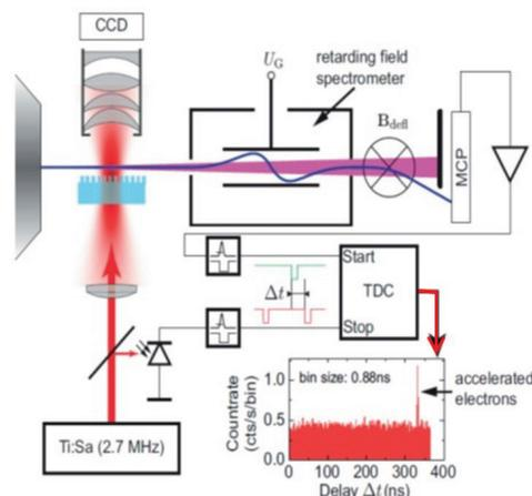
Figure 3: The coincidence circuit used to detect a correlation in the integrated MCP count rate with the arrival time of the laser pulse.
