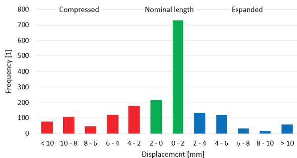
Figure 3: Length deviations of LHC warm modules.
