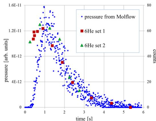
Figure 2: Benchmarking dynamical Molflow+ with the beta scintillators, for  $^6\text{He}$ . Units are arbitrary.
