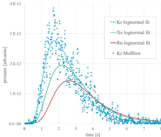
Figure 3: Arrival time distribution calculated with Moflow for Kr, Xe and Rn for a square pulse of gas generated at the transfer line entrance. For simplicity, only the lognormal fit is displayed for Xe and Rn.
