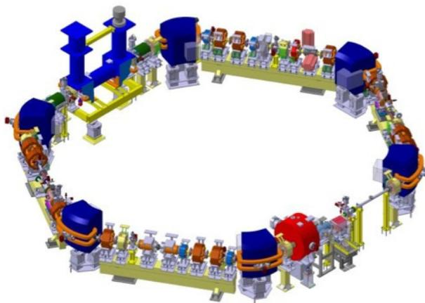
Figure 3: ELENARing components, with “U”-shaped electron cooler (EC) visible on the left (in blue), and cylindrical injection kicker tank (in red), lower right.
