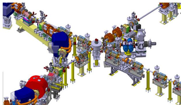
Figure 2: a busy crossing; the ion-switch (IS) chamber is in the middle, with its 5 connections to, clockwise from the 2-hour position: LNI from AD, LNS, LNE03, LNI going into LNR, and LNE00 coming out of the ring.
