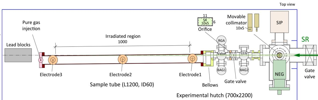
Figure 1: Experimental setup.
