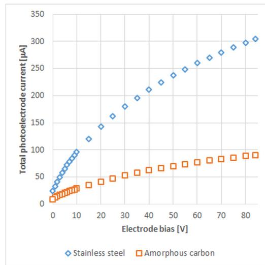
Figure 3: Photoelectron currents at different bias voltages for the stainless steel and amorphous carbon samples, at the beginning of the conditioning.
