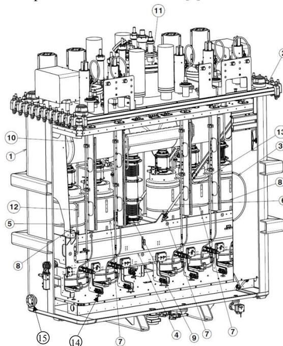
Figure 1: The complete HIE-ISOLDE high- $\beta$  cryo-module; 1 Vacuum vessel lower box, 2 Vacuum vessel top plate assembly, 3 Thermal shield lower box, 4 Support frame, 5 Suspension end plate, 6 Tie-rod, 7 Inboard cavity, 8 Outboard cavity, 9 Down tube to solenoid, 10 Helium vessel, 11 Chimney assembly, 12 Support frame cooling supply, 13 Support frame cooling return, 14 Mathilde targets, 15 Mathilde viewport.
