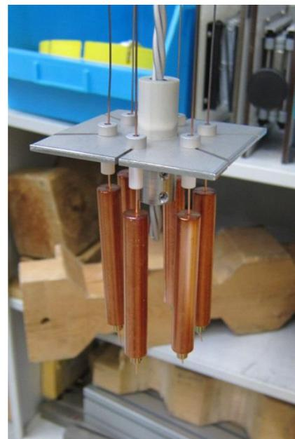
Figure 4: Centring plate and weights for the anodes
