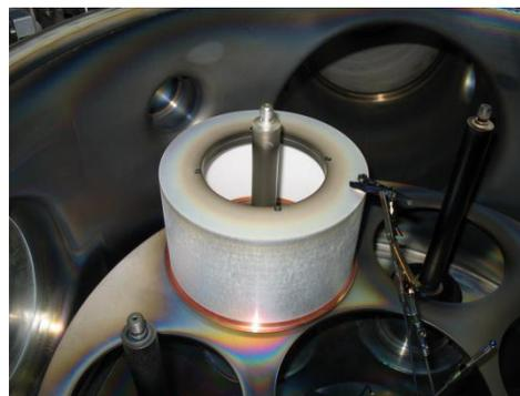
Figure 1: Cylindrical coating configuration for high resistivity coating of RF ceramic windows.
