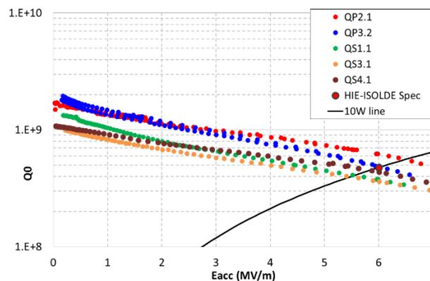
Figure 2: RF test results of the 5 cavities of the first cryomodule.
