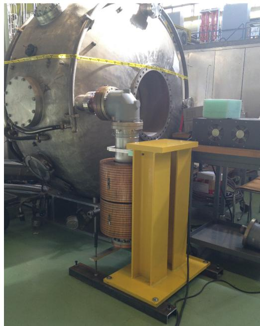
Figure 2: Picture of the mock-up 88 MHz cavity used for testing of the tuning-concept with the fast ferrite tuner.
