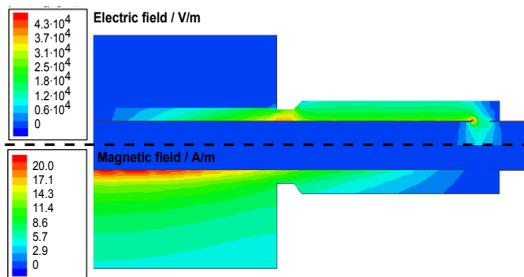
Figure 6: Preliminary design of accelerating cavity. Top: electric RF field distribution, bottom: magnetic RF field distribution for  $\mu' = 8$ .
