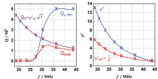
Figure 5: Left:  $Q_{\text{total}}$ ,  $Q_{\mu, \text{ferr}}$  and  $Q_{\Omega}$  vs. frequency. Right:  $\mu'$  and  $\mu'_{\text{eff}}$  vs. frequency.
