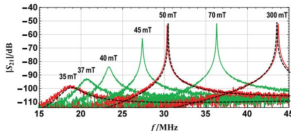
Figure 2: Measurement results (solid traces) of resonant ferrite filled setup in comparison with driven modal simulation results (dashed traces).
