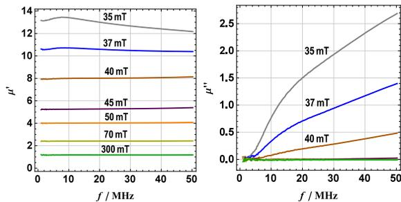
Figure 4: Measured complex permeability vs. frequency for different magnetic bias fields.
