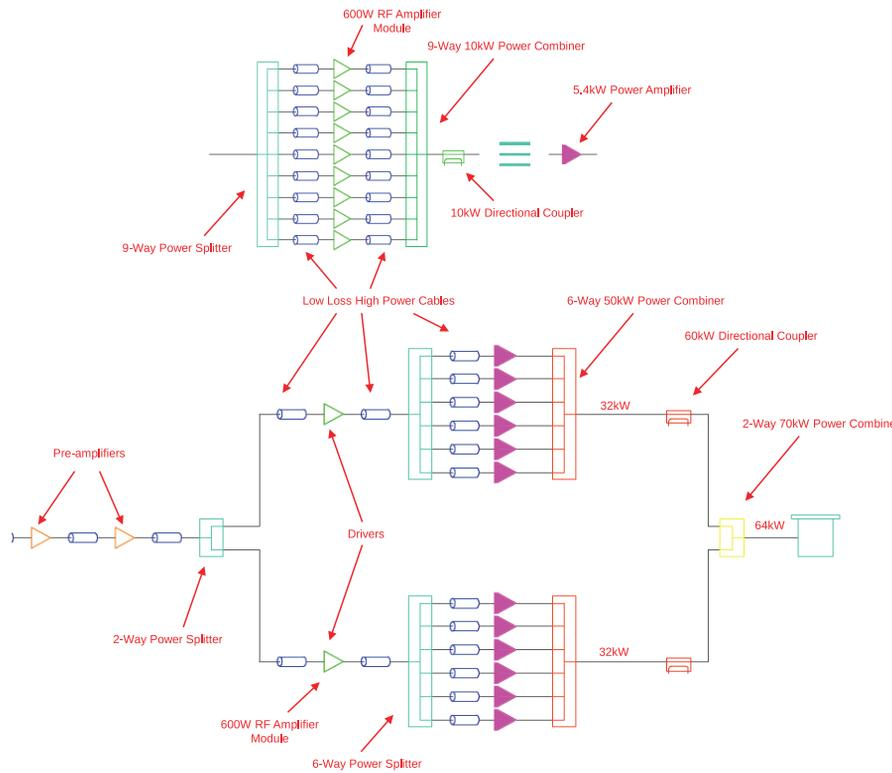
Figure 1: Block diagram of 65 kW 500 MHz amplifier system.
