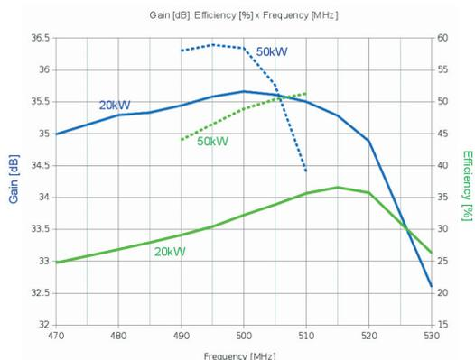
Figure 5: 65 kW system: Gain vs. Frequency.
