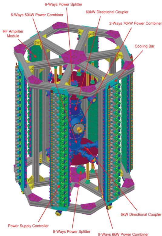
Figure 2: 3D View of 65 kW 500 MHz amplifier system.
