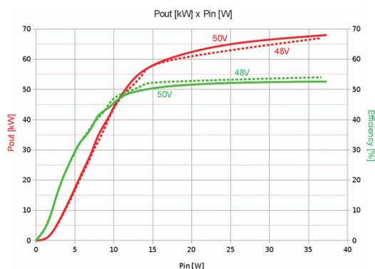
Figure 4: 65 kW system:  $P_{out}$  and Efficiency vs.  $P_{in}$ .
