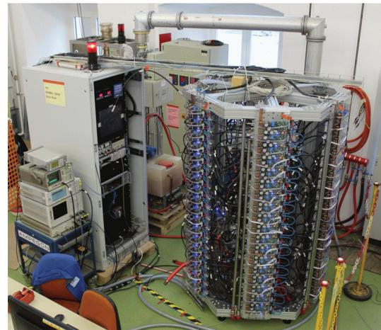
Figure 3: The complete 65 kW solid-state power amplifier (SSPA) in operation and delivering  $P_{out} = 64\text{ kW}$
