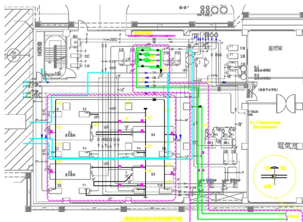
Figure 2: Chilled water piping in the Utility Building II.
