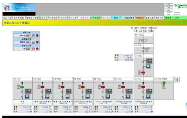
Figure 3: Feeder A of the TPS SCADA.
