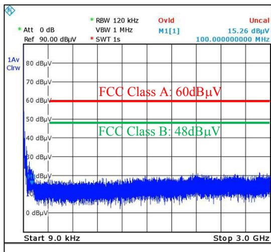
Figure 7-2: Conducted EMI for 100 V firing.
