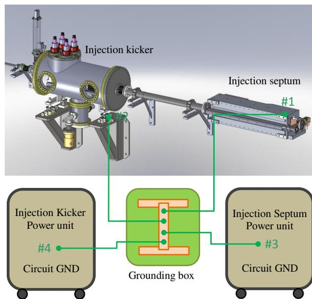
Figure 2: TPS injection pulsed magnets grounding scheme.
