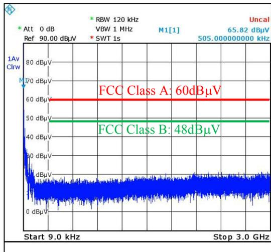
Figure 7-1: Conducted EMI for system Standby.
