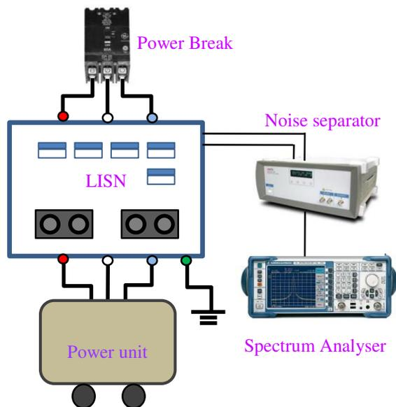
Figure 6: Experimental setup for conducted EMI measurement.
