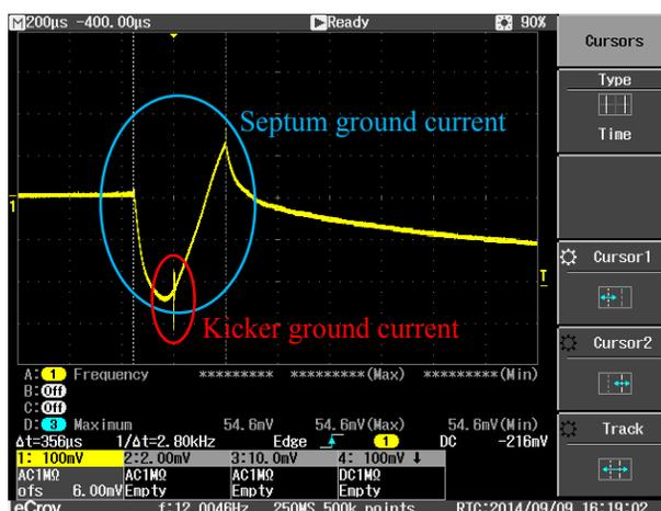
Figure 5: Grounding current (#4) for kicker and septum fire simultaneously.
