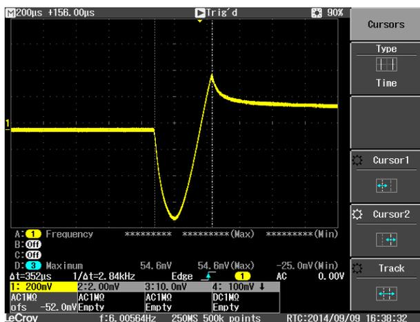
Figure 3: Grounding current (#1) for septum fire.
