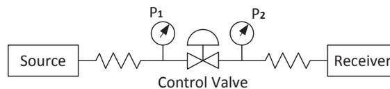
Figure 7: Typical installation of a control valve.
