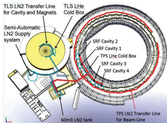
Figure 2: Configuration of LN<sub>2</sub> transfer line of NSRRC.
