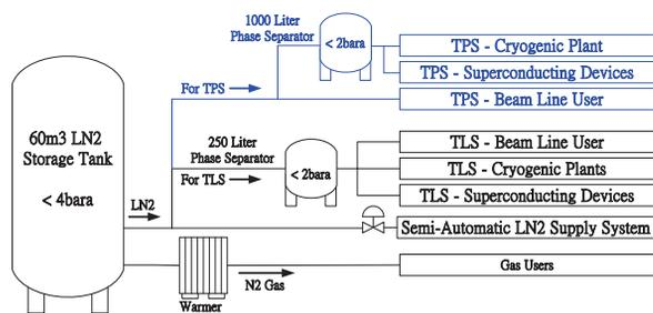
Figure 1: Configuration of the LN<sub>2</sub> supply system at NSRRC.
