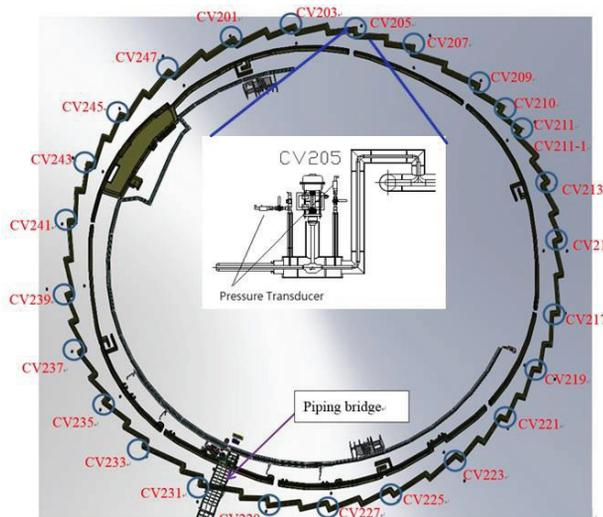
Figure 6: Overall transfer line for beam-line at TPS.
