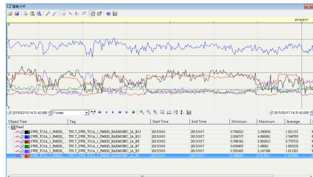
Figure 6: The 3<sup>rd</sup>, 5<sup>th</sup>, 7<sup>th</sup>, 9<sup>th</sup>, 11<sup>th</sup> and 13<sup>th</sup> order harmonics after installing the filters.
