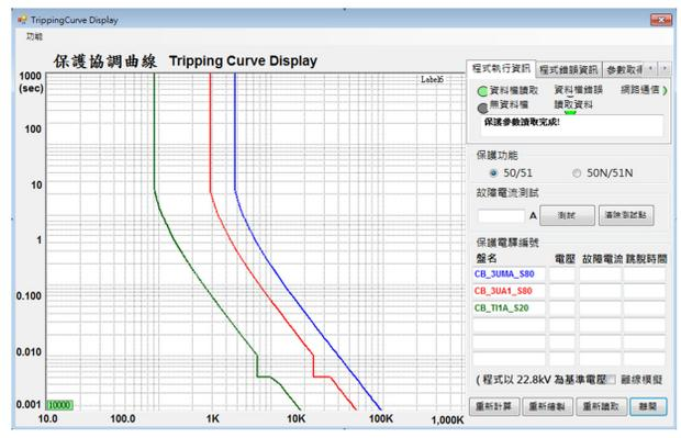
Figure 9: A tripping curve display of feeder A.
