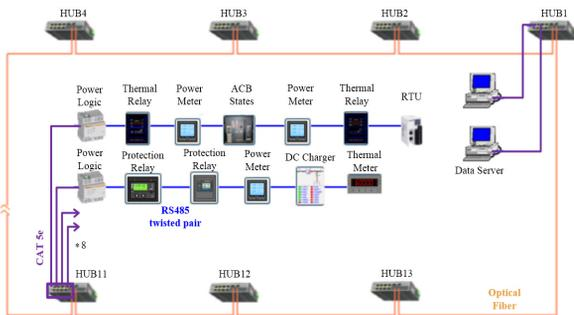
Figure 3: The communication architecture of SCADA.
