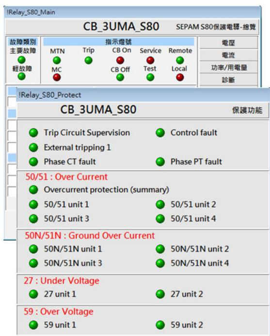
Figure 8: The status of protection relays.
