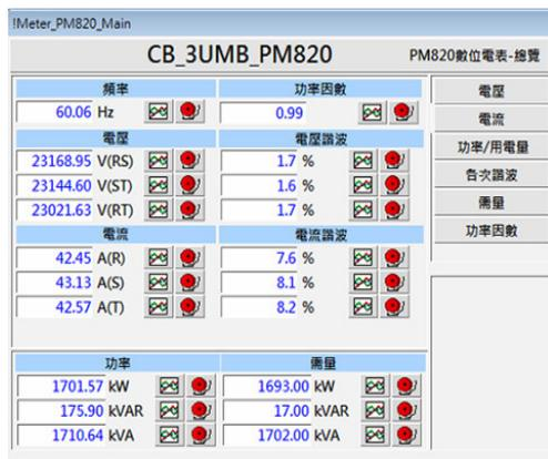
Figure 4: The real time information of feeder B measured by the power SCADA system.
