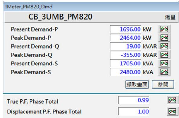
Figure 5: The power demands and the power factor at the time of measurement, and also the historic peak value.
