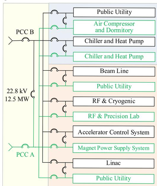
Figure 1: Block diagram shows the loads used at TPS.
