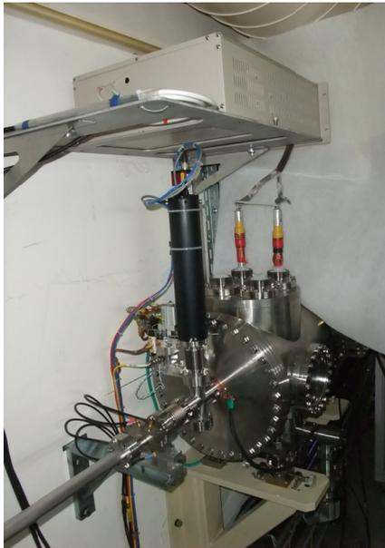
Figure 5: The field testing LTB kicker pulser and magnet.
