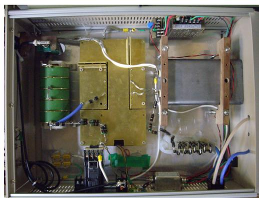
Figure 4: The layout of IGBT test unit circuitry.
