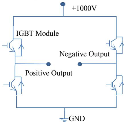
Figure 3: Topology of the dipole power supply.
