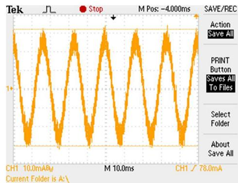
Figure 5: Using the positive output line and ground line of the AC source connection to measure the current.
