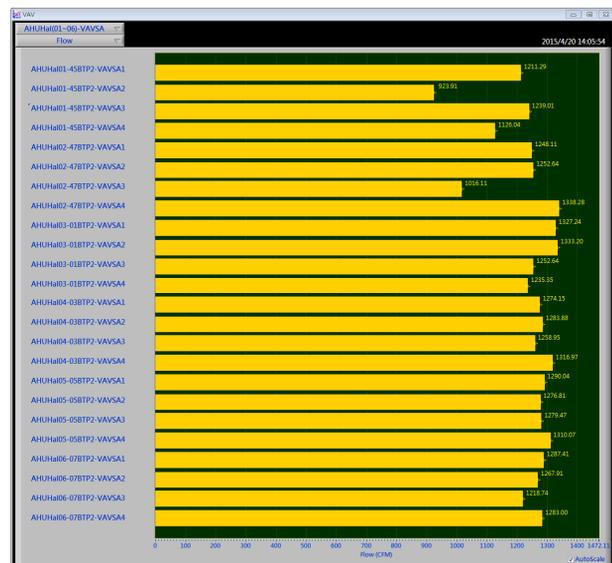
Figure 8: TAB information of the HVAC system.
