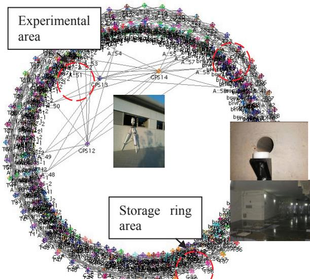
Figure 4: The survey network of TPS.
