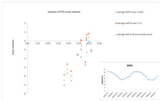
Figure 6: The Variation in radial direction with temperature.
