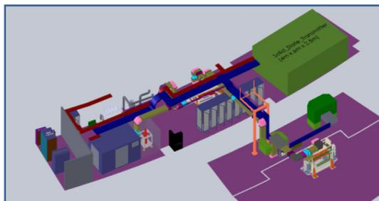
Figure 2: Arrangements of signal (blue) and AC-power (red) trays are set as a double layer in the controller area, but as a single layer in the loading area (blue).
