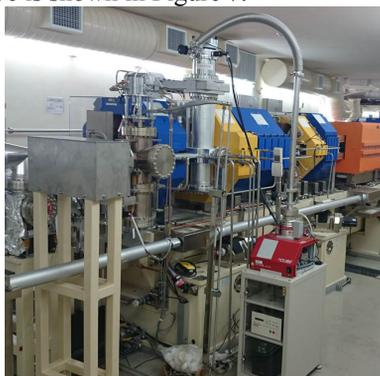
Figure 7: The exhaust pumping system in TPS storage ring.
