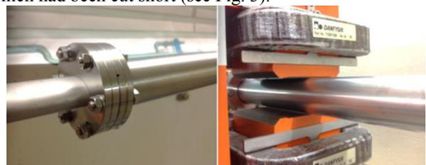
Figure 3: Left: elliptical chamber connected with circular chamber. Right: circular chamber goes through booster corrector magnet.
