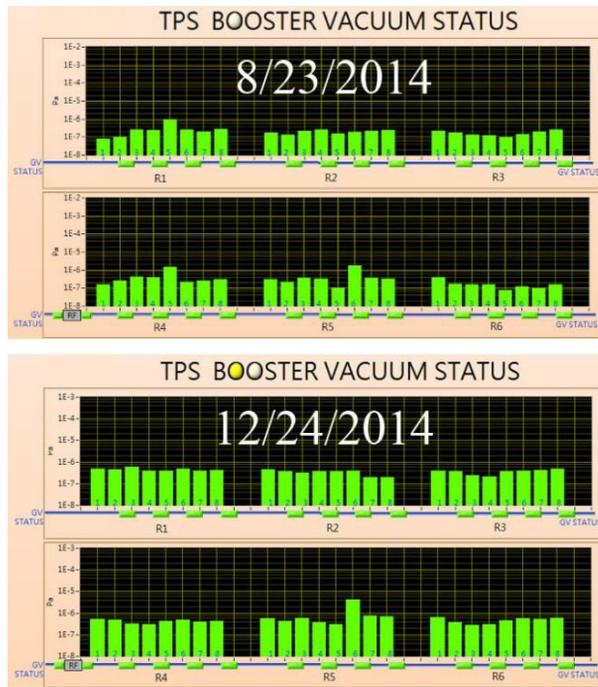
Figure 5: Booster vacuum pressure before and after demagnetization.
