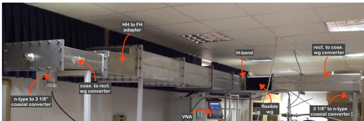
Figure 5: Assembled transmission line of the SPP.
