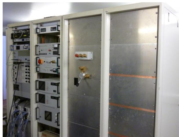
Figure 4: TDC klystron modulator.
