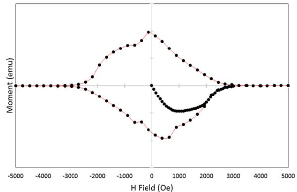
Figure 7: Magnetic hysteresis loop  $M(H)$  for film C deposited onto polycrystalline Cu.  $H_{C1} = 1076$  Oe and  $H_{C2} = 3205$  Oe.
