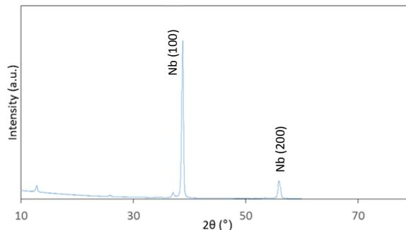
Figure 5: Nb (110) and (200) grown on polycrystalline Cu by HiPIMS with -100 V DC bias. Average grain size is 24 nm.
