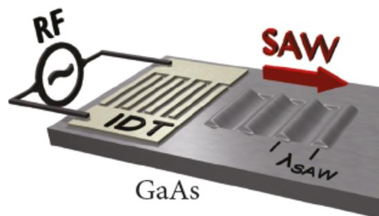
Figure 1: Generation of SAW on a piezoelectric substrate with an interdigital transducer (IDT) powered by an RF-source.
