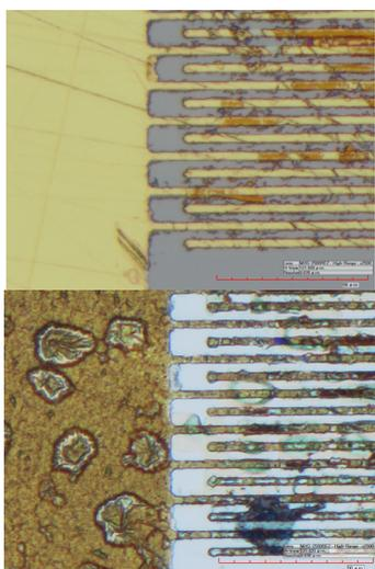
Figure 3: IDT device on GaAs substrate before (upper picture) and after (lower picture) heat processing at about  $550\text{C}$  [10].
