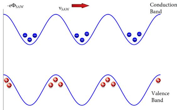
Figure 2: Band distortion, dynamical formation of type-II band structure in GaAs and charge carrier separation under piezoelectric potential  $\Phi_{SAW}$  of propagating SAW.
