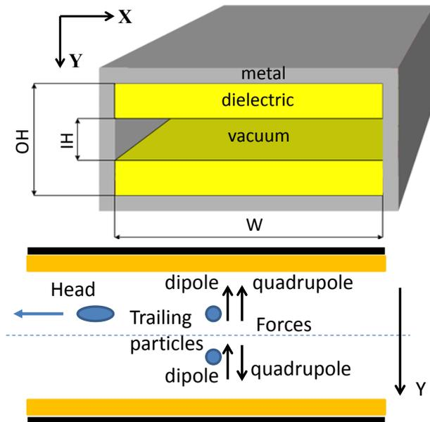
Figure 3: DWA based on a rectangular dielectric-lined waveguide (top). Deflecting forces acting on trailing particles in the rectangular DWA (bottom).
