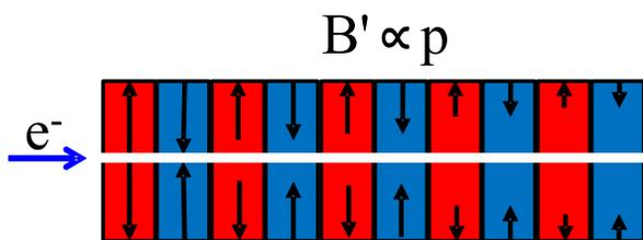
Figure 1: FODO lattice with the magnet strength linearly decreasing towards higher propagation distances.
