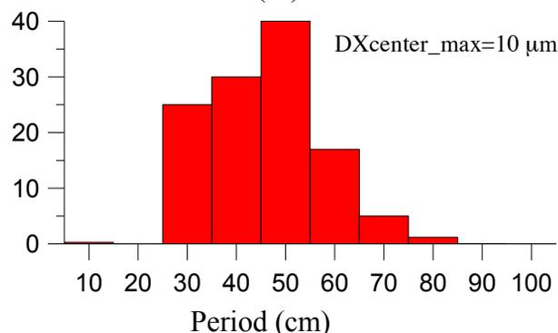
Figure 2: Simulated particle loss for different bending periods which are whole numbers of decimeters.
