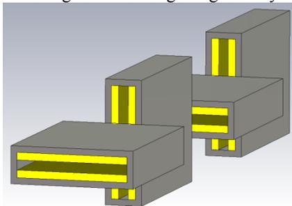
Figure 4: Configuration with an alternating quadrupole field.
