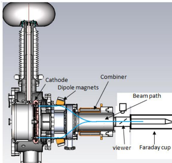
Figure 1: Schematic diagram of the gun.
