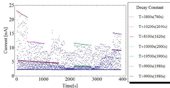
Figure 7: Two beam operation decay curve.
