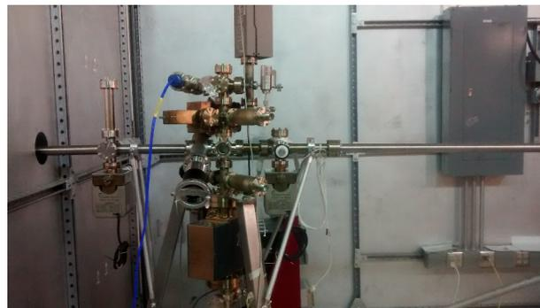
Figure 2: The transfer line, cathode preparation chamber and long manipulator, as shown from left to right.
