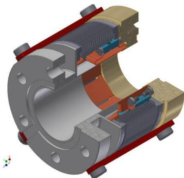
Figure 7: Section view of the bellows. Axial compression/expansion limits are 10/1.5 mm. No lateral movement is allowed. Free length is 50 mm.
