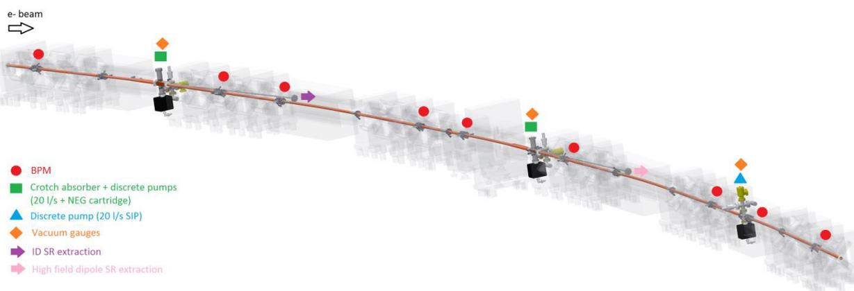
Figure 2: Vacuum system layout for one achromat cell.
