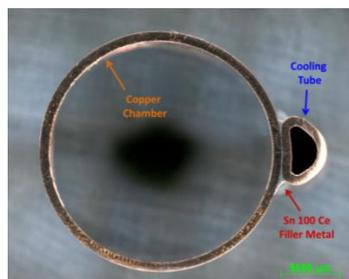
Figure 4: Multipole vacuum chamber cross section with the vacuum soldered special shaped cooling tube.
