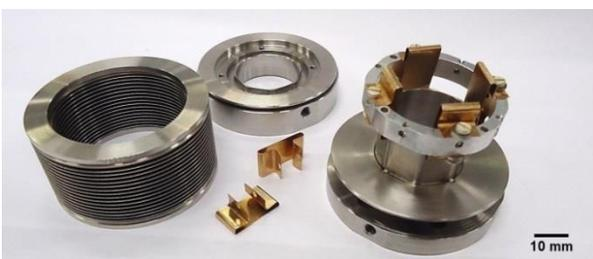
Figure 8: View of the main parts of the bellows.
