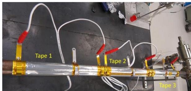
Figure 9: Three heaters assembled on a copper vacuum chamber for NEG activation test.
