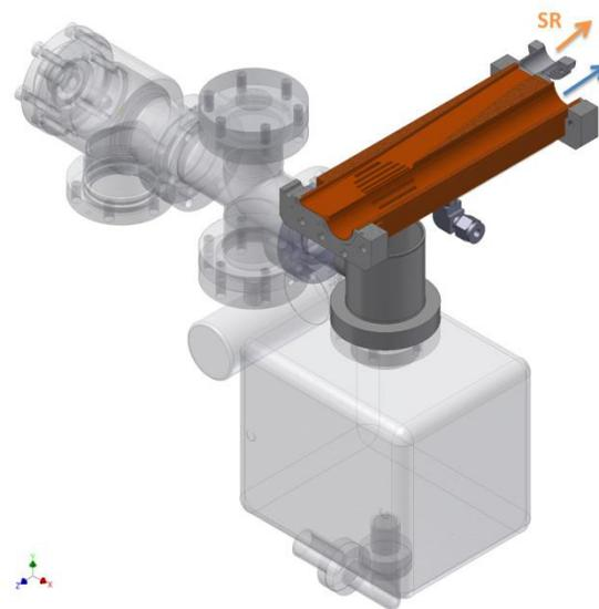
Figure 5: Crotch absorber with a radiation extraction port.
