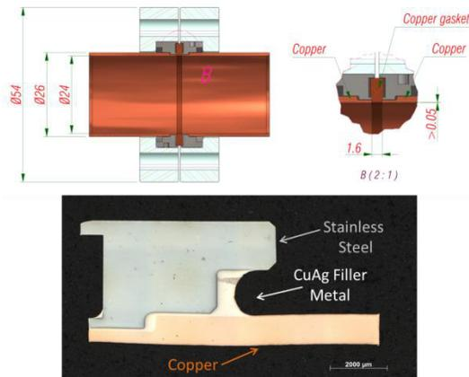
Figure 3: Section view of a circular vacuum flange assembly (top) and section cut of an as-brazed flange (bottom).
