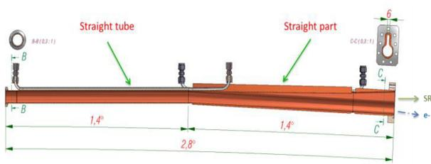
Figure 6: Section view of the dipole vacuum chamber with narrow antechamber for IDs radiation extraction. Fabrication is based on two straight sectors permitting to protect the small thickness tube sector from wigglers high power loads.
