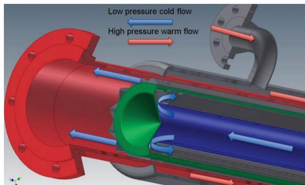
Figure 4: Sub-atmospheric heat exchanger [6].
