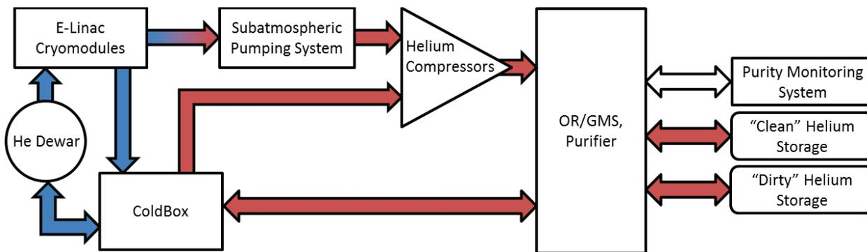
Figure 1: Architecture of the e-linac cryogenic system.
