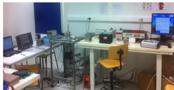
Figure 2: (a) Scheme and (b) View of the Coaxial resonator multipacting test bench.
