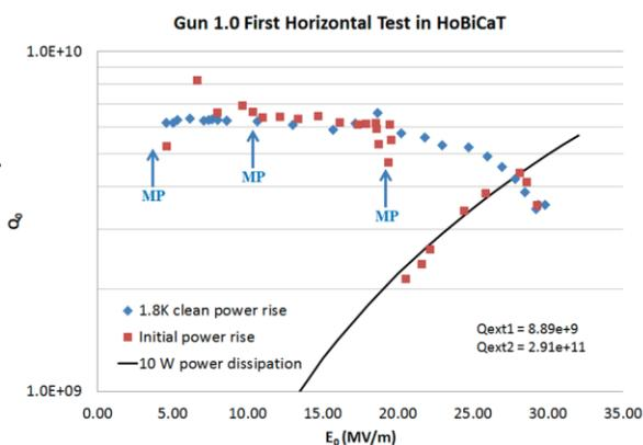
Figure 5: The first test results obtained for Gun 1.0 in HoBiCaT using the same RF coupler configuration as was shipped from JLab.
