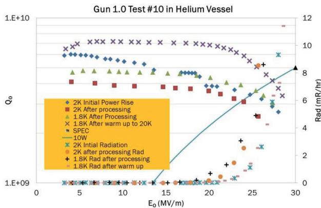
Figure 3: The vertical RF test results from the JLab VTA at 1.8 and 2K for the cavity in the helium vessel. The accelerating field  $E_0$  is the peak on axis electric field, the most relevant measure for a photoinjector.
