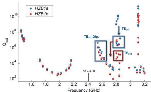
Figure 2:  $Q_{ext}$  calculations on the models loaded with standard beam-pipes. Standard beam-pipe+standard WG-D (87mmx50mm), HZB1. Standard beam-pipe+extended WG-D (87mmx60mm), HZB1b.
