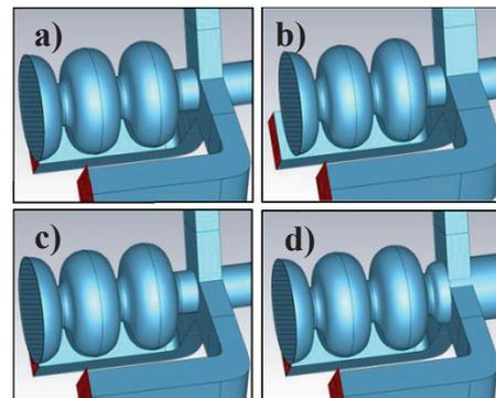
Figure 1: Layout of the two techniques applied on the optimization of the Y-shape waveguide absorbers. Extended WG-D (a~b). Enlarged beam-pipe (c~d).
