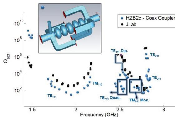
Figure 4: Layout of the HZB 1.5 GHz prototype model loaded with WG-D and coaxial FPC. Enlarged beam-pipes are used ( $\phi=110$ mm) (a). Comparison between the “HZB2c-coax coupler” model after tuning with respect to the JLAB “High current” simulation results (b) [10].
