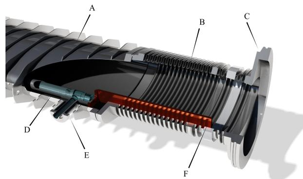
Figure 4: Outlet side of the beam pipe. A: Oval beam pipe, B: Metal bellow, C: Flange, D: Water cooling pipe, E: Water feedthrough, F: Copper heat sink
