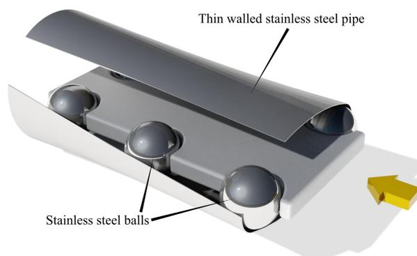
Figure 1: Schematic representation of the bending process to form the round feedstock into the required oval shape.
