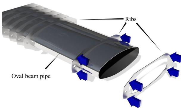
Figure 2: Mounting and positioning of the ribs.
