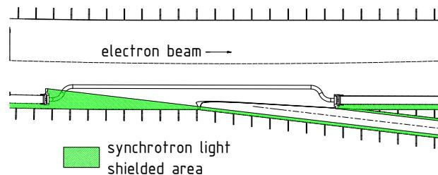
Figure 6: Sectional view of the sideways branch with synchrotron radiation shielding.
