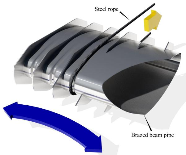
Figure 3: Pipe constriction and bending.
