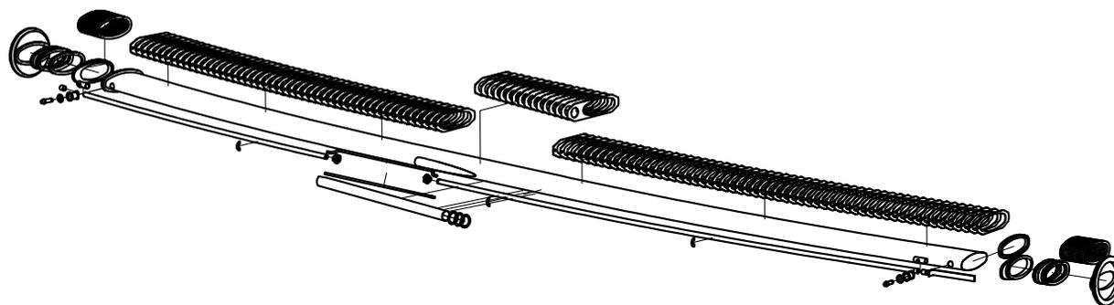
Figure 5: Exploded drawing of a beam pipe with sideways branch and all single parts.
