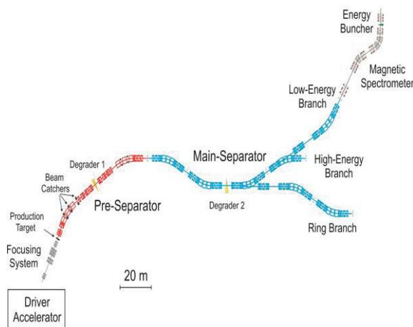
Figure 1: Magnetic Layout of Super-FRS.
