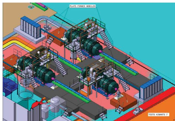
Figure 4: Sketch of the test station at CERN (with a long multiplet installed at all three benches).
