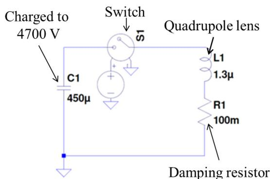
Figure 1: LTSpice[2] model of the electrical circuit of the prototype. The circuit is nearly critically damped to avoid oscillations.
