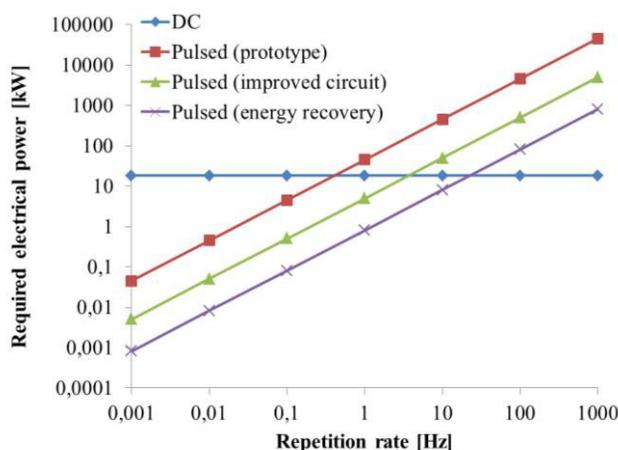
Figure 8: Power saving depending on the repetition rate of the pulsed lens.
