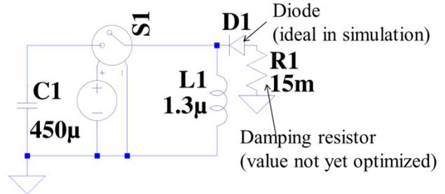
Figure 5: Improved circuit for quadrupole lens, LTSpice [2].
