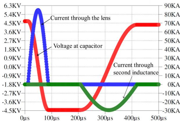
Figure 7: Results of the circuit simulation shown in Fig. 6.
