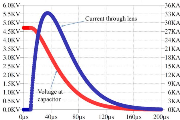
Figure 2: Pulsed current and voltage (Result of simulation in Fig. 1).
