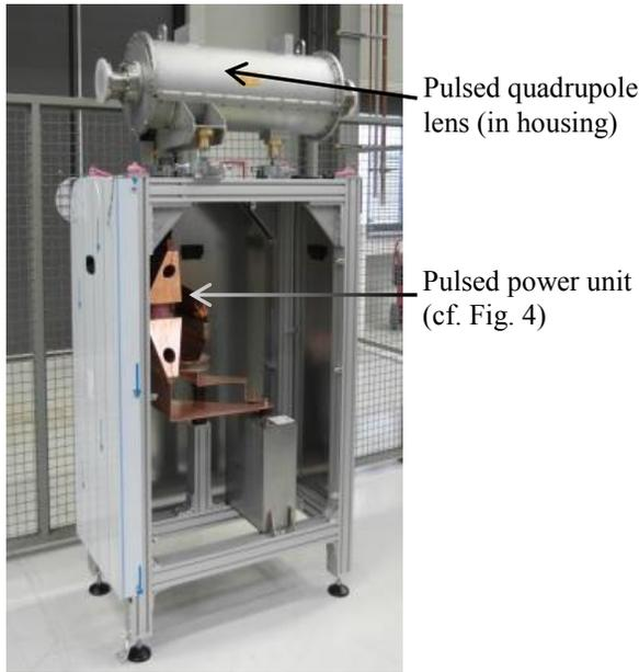
Figure 3: The prototype of the pulsed quadrupole lens. The pulsed power unit is situated below the lens.
