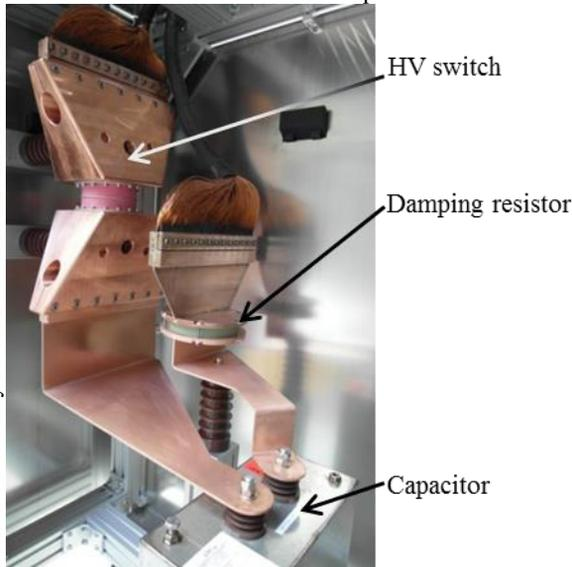
Figure 4: Pulsed power of the prototype.
