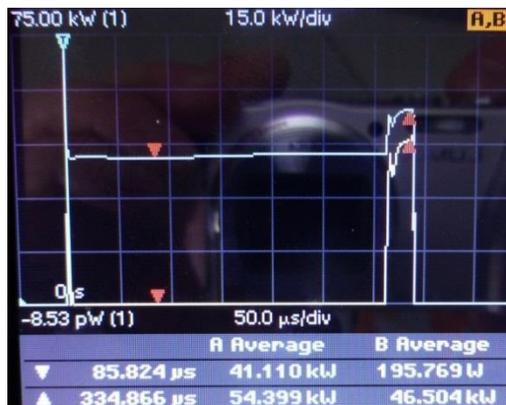
Figure 5: A discharge leads to amplifier shutdown.
