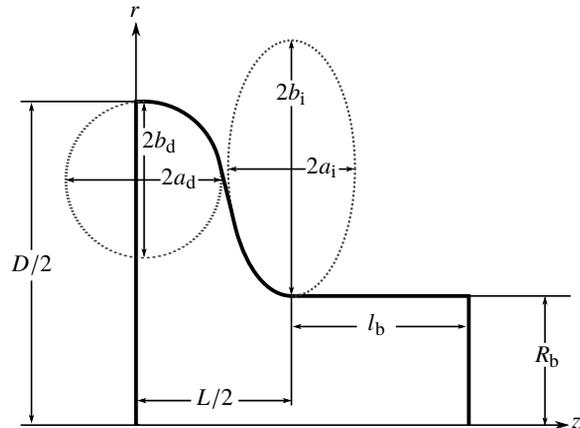
Figure 1: Geometry parameters of an elliptical cavity.
