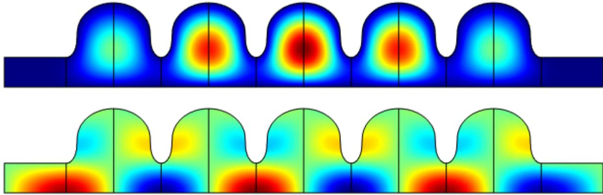
Figure 2: Cross section view of the electric field distribution of the TE<sub>011</sub> (top, out-of-plane electric field) and TM<sub>021</sub> mode (bottom, electric field in beam direction).
