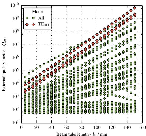
Figure 6: External quality factors of all cavity and normal modes with a fixed phase advance of  $\psi = \frac{\pi}{2}$  as a function of the beam tube length  $l_b$ .
