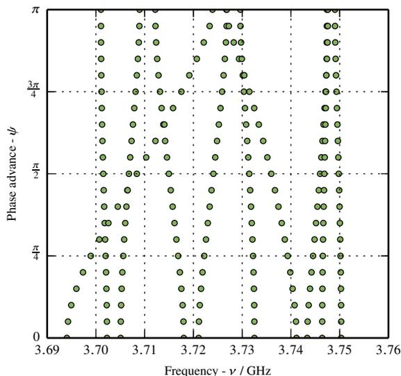
Figure 5: Dispersion relation of the cavity mode 6 and a waveguide mode. Both passbands overlap.
