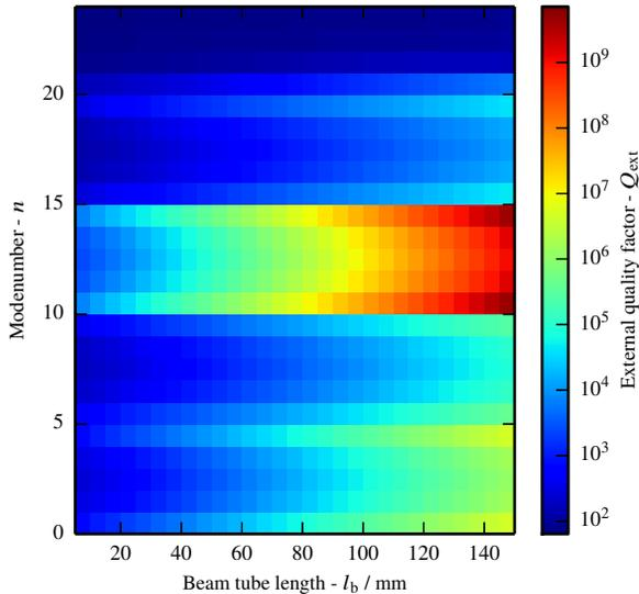
Figure 3: External quality factors  $Q_{\text{ext}}$  for the first 5 cavity modes and their corresponding normal modes as a function of the beam tube length  $l_b$ .
