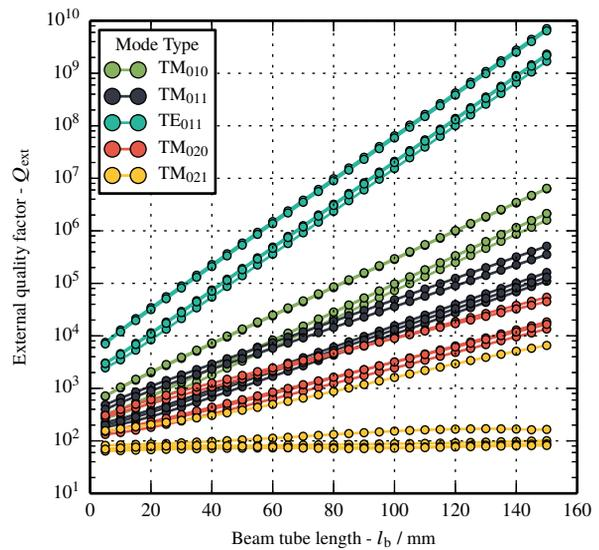
Figure 4: External quality factors  $Q_{\text{ext}}$  for the first 5 cavity modes and their corresponding normal modes as a function of the beam tube length  $l_b$ .
