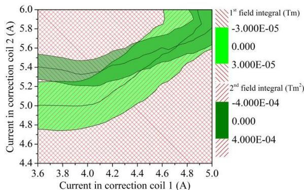
Figure 6: Color plot of the 1<sup>st</sup> and 2<sup>nd</sup> field integrals for different correction coil currents.
