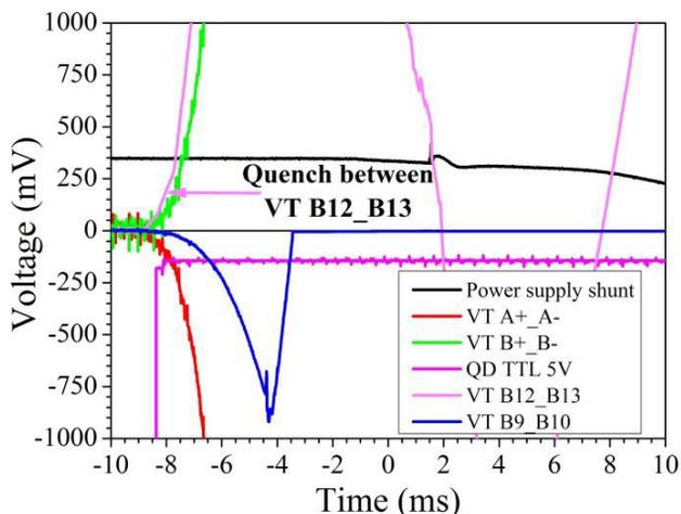
Figure 2: Typical voltage behaviour during a quench.
