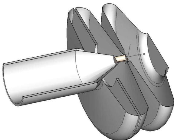
Figure 9: Large split choke-cells tuned to 1.3 GHz.
