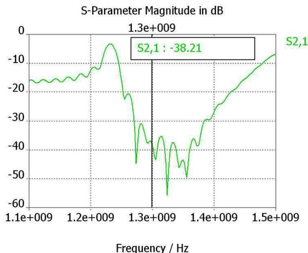
Figure 10:  $S_{21}$ -parameters of large split choke-cells.
