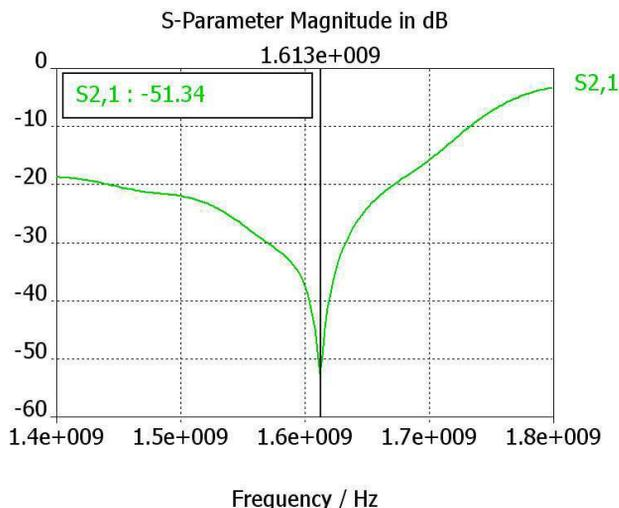
Figure 3: Typical  $S_{21}$ -parameter frequency dependence of 1.4- and choke-cell structure ( $z_{\text{choke\_gap}} = 21.5$  mm).
