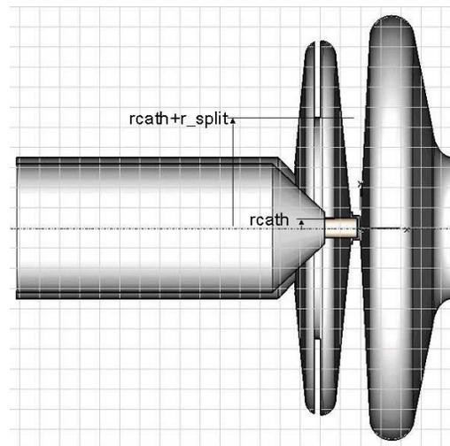
Figure 5: Split choke-cell simulation model.
