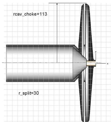
Figure 7: Split choke-cell notch filter tuned to 1.3 GHz.
