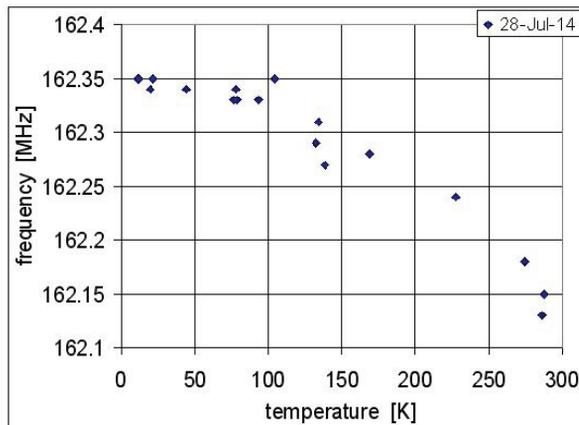
Figure 7: Frequency change during cavity cool-down.
