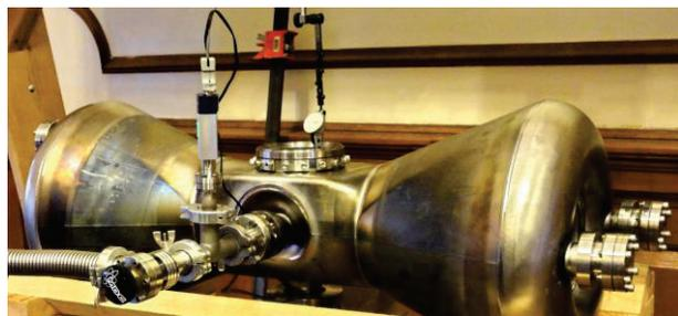
Figure 1: Modified cHWR with leak check setup.
