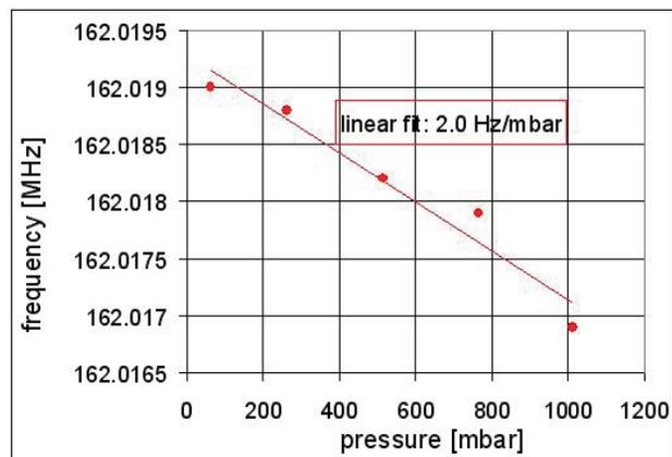
Figure 6: Frequency shift during helium vessel leak test.
