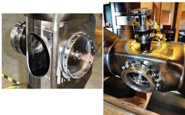
Figure 4: Cavity tuner section.
