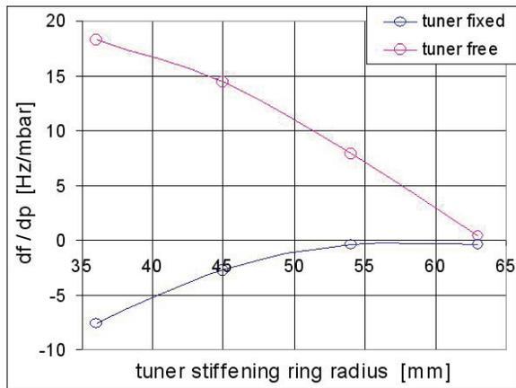
Figure 3: cHWR tuner ring position optimization.
