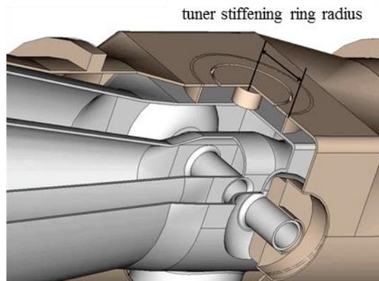
Figure 2: cHWR simulation model central part.
