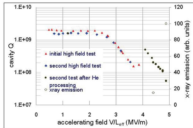
Figure 9: Q measurements at 4K.
