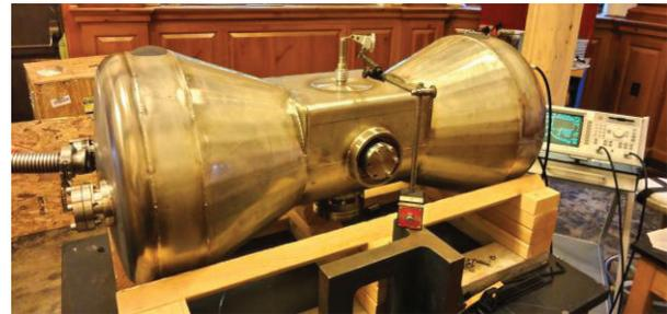
Figure 5: Helium vessel leak check setup.
