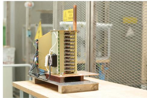
Figure 4: The solid-state switch being prepared for installation in the spare modulator.
