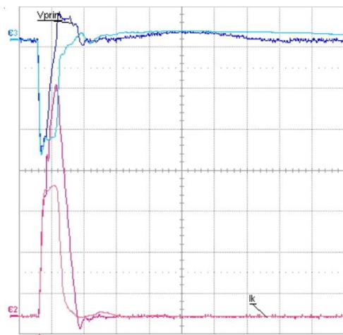
Figure 3: Klystron voltage (blue) and current (purple) after circuit modification. Darker colours show the curves in case of an arc.
