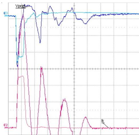
Figure 2: Klystron voltage (blue) and current (purple) before circuit modification. Darker colours show the curves in case of an arc.
